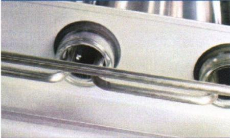
The pipes are mass produced with just a minimum numbering of soldering points. This results in high leakage safety and a reduction of internal scaling.
